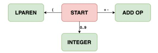
The machine should have a single starting state (the START state). The machine's transitions depend on the value of the next character. For example, given the input 123, we would start in the START state and then the 1 at the start of the input would cause a transition to the INTEGER state. Clearly the INTEGER state is not complete, as is it has no way to add the remaining digits (2 and 3) to the integer being created.
